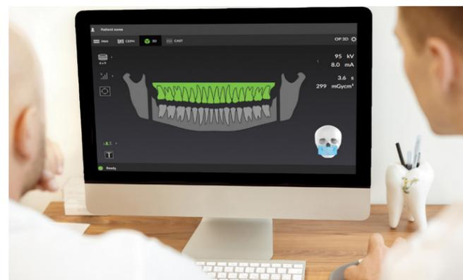
The desired imaging area can be selected intuitively with the ORTHOselect user interface. Selections can be made as individual teeth, an entire upper or lower jaw, or TMJ. The optimum field-of-view (FOV) is set automatically based on the selection.
